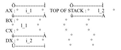
Note: i\_2 is placed in DX and I\_2 on the stack. When the compiler processes I\_2 there is no register pair remaining for the long, 32-bit, value I\_2, therefore it is pushed on the stack. However, when the compiler reaches i\_2 (a 16-bit value), it puts this value in DX because this has not already been used.
